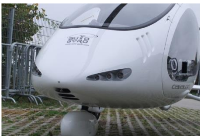
Air intake and gills for condenser
